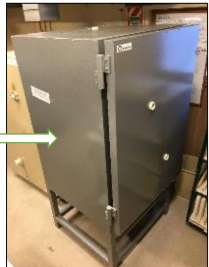
**FE2** has blown its bottom elements – it has limped through a few bisques but will be out-of-action until the new elements arrive.
